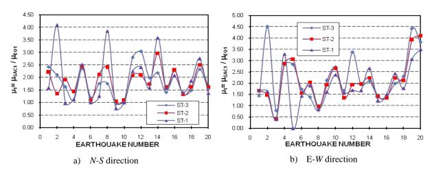
Fig. 3. Values of the  $\mu_1$  parameter, 3-level building elastic behavior
