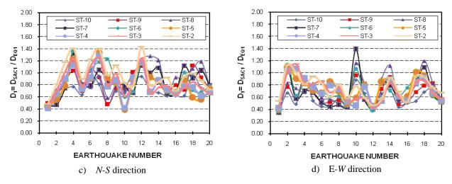
Fig. 2. Values of the  $D_1$  parameter, 10-level building elastic behavior
