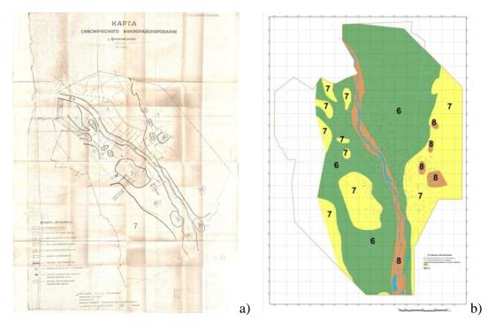
Figure 1. The map of seismic microzonation of 1970: original (a), GIS-project (b)
