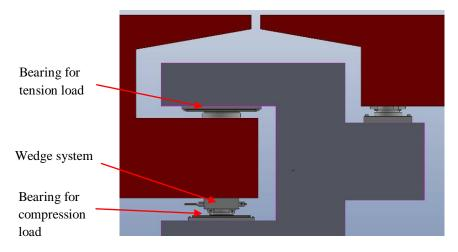
Figure 4. Spherical bearings coupled to carry both compressive and tensile vertical load
