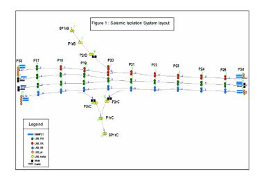
Figure 7. Bearing and isolation system for the link PS3-PS4
