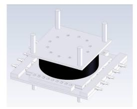
Figure 8. LRB with guided sliding plate able to allow only irreversible movements
