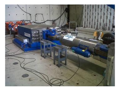
Figure 11. Viscous damper FD 3750/550 during the tests
