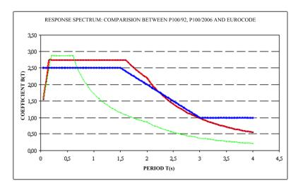
Figure 2. Comparison between response spectra of Bucharest given by P100-92 (bleu), P100\_1/2006 (red) and Eurocode 8 (green)
