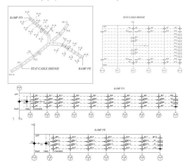
Figure 3. Bearing layout stay cable bridge
