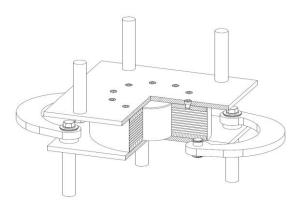
Figure 10. LRB coupled with transversal hysteretic C-shaped elements for the ramps of PS3-PS4
