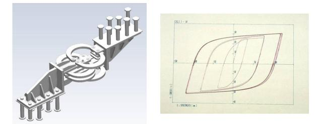
Figure 6. Hysteretic device installed on the ramps abutments and typical force-displacement loop
