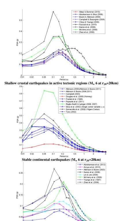
**Figure 3.** Predicted elastic pseudo-acceleration response spectra from for a rock site for (top): a strike-slip shallow crustal earthquake of Mw 6 at a distance to the surface projection of the rupture of 20km, (middle): an Mw 6 earthquake in a stable continential region at a distance to the surface projection of the rupture of 20km, and (bottom): an Mw 6.5 interface earthquake in a subduction zone at a rupture distance of 50km.
