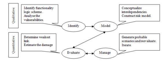
Figure 3.2. Fault-tree analysis process
