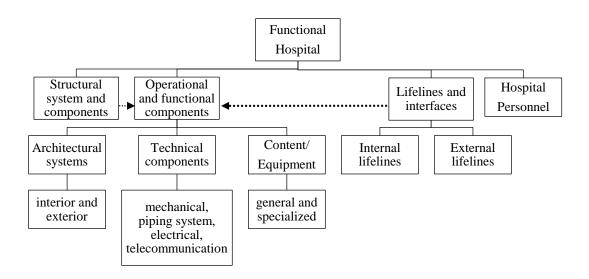
Figure 3.1. Functional components of a hospital
