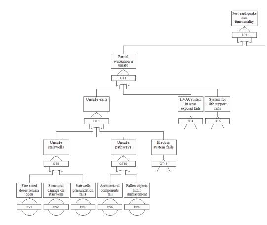
Figure 5.1. Fault tree for "unsafe partial evacuation"
