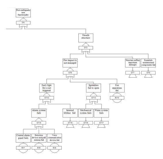
Figure 5.2. Fault tree for "unsafe structure"
