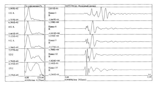
Fig. 3. Occurrence of a significant HF component in the near field of a powerful non-explosive pulsed source of GSK-6M
