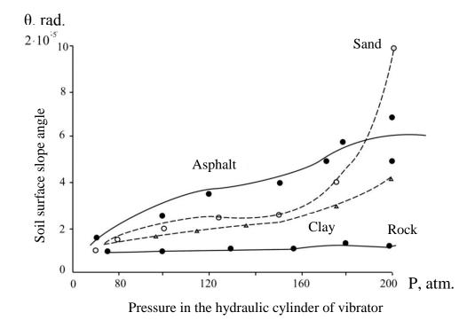
**Figure** 7. The effect of pressure in the hydraulic cylinder of the vibrator on seismic radiating effect of soil slope from the distance to the source (P. Uznozh, Belarus, 1992; city Dedoplistskaro, Georgia, 1992)
