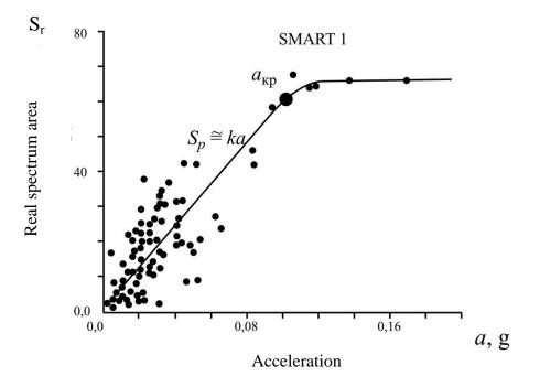
Figure. 4. The dependence of the real spectrum area from acceleration (Taiwan)
