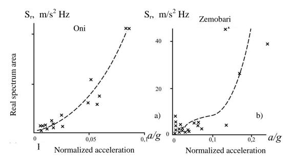
Figure5. The dependence of the real spectrum area of vibrations from acceleration SMACH (Georgia, 1991)
