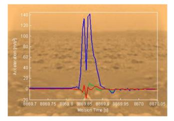
Figure 2. Data of "Huygens Spacecraft" accelerometer while landing on Titan's surface The landing speed was equal to 4.6 m/sec [site <u>www.esa.int</u>].
