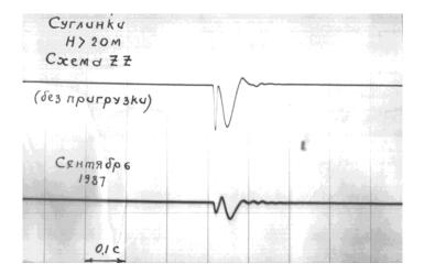
Figure 1. Nonlinear phenomena in soft soils under intense seismic loads
