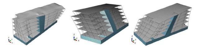
Figure 4. Building II; 1<sup>st</sup> Mode 1.44Hz (left), 2<sup>nd</sup> Mode 2.17Hz (mid), 3<sup>rd</sup> Mode 2.82Hz (right)
