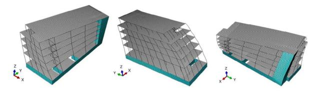
Figure 3. Building I; 1<sup>st</sup> Mode 1.45Hz (left), 2<sup>nd</sup> Mode 2.16Hz (mid), 3<sup>rd</sup> Mode 3.45Hz (right)
