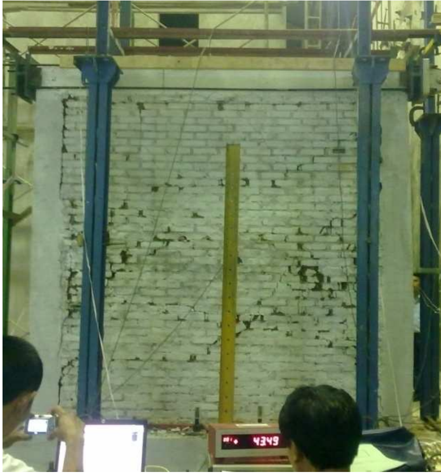
Figure 5. Damages observed during the test of specimen 1.
