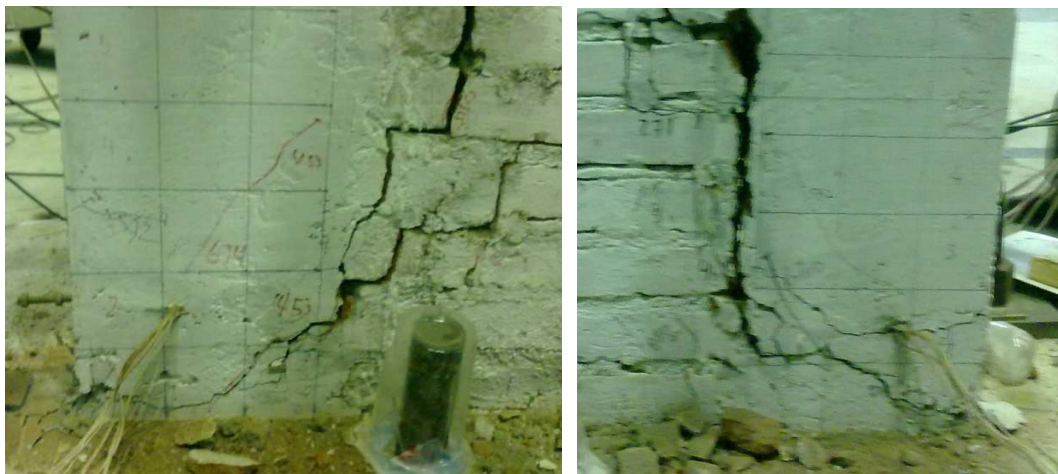
Figure 6. Damages observed at the corners of the concrete frame during the test of specimen 1
