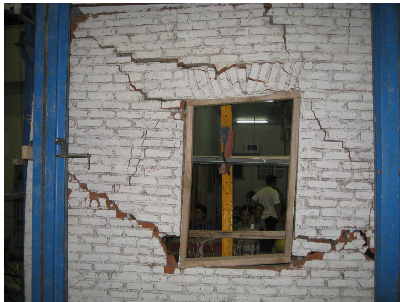
Figure 8. Damages around window frame of specimen 2 near the end cycle of test
