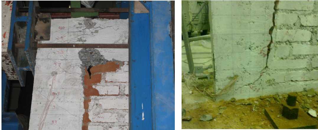
Figure 7. Damages observed at the corners of the concrete frame during the test of specimen 2
