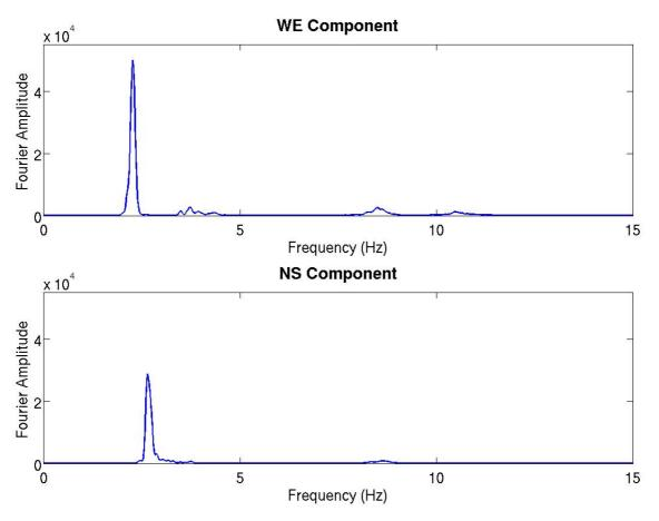
Figure 2. Example of rotational HVSR analysis for building nº 44
