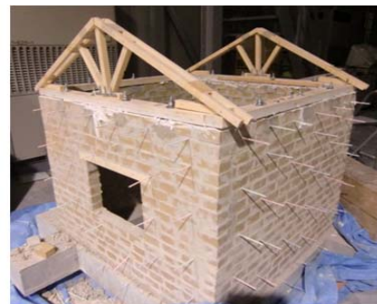
2. Securing holes using the straw during model construction
