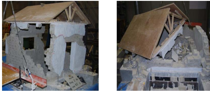
Figure 5. Non-retrofitted building model after 46 run (left) and 47 run (right)
