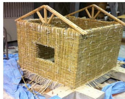
4. Connecting inner and outer meshes by PP strings and overlapping the meshes around the opening & roof
