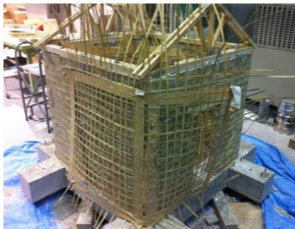
3. Wrapping the building from inside and outside by the mesh
