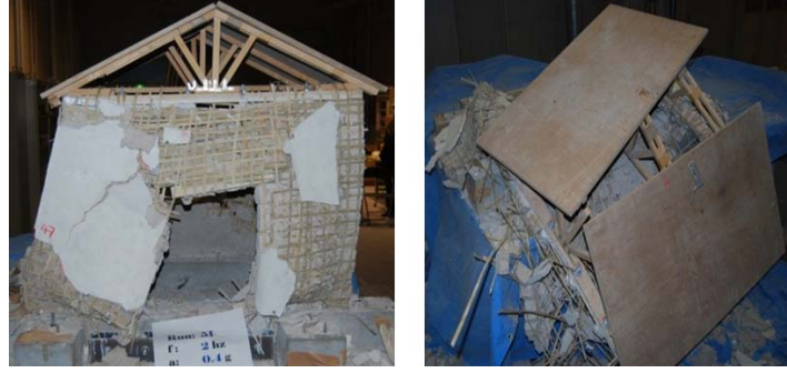
Figure 7. Retrofitting building model after 51 run (left) and 52 run (right)
