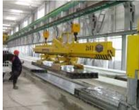
Figure 3. Automated line for production of reinforced concrete extrusion-type slabs by Finish technology at Sevastopol “CONSOL LTD”
