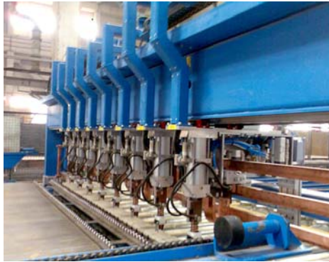
Figure 3. Automated line for production of reinforced concrete extrusion-type slabs by Finish technology at Sevastopol “CONSOL LTD”
