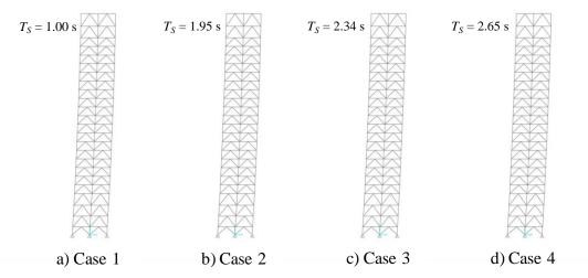
Figure 4. Fundamental mode of vibration due to global shear drift mode for all versions of bracing system
