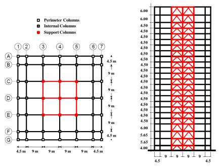
Figure 2. Geometry and structural layout of braced twenty four-story building
