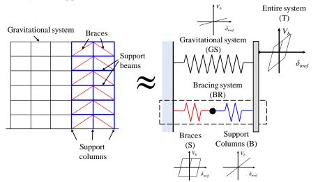
Figure 1. Modeling assumptions for tall buildings stiffened with a bracing system
