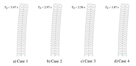
Figure 5. Fundamental mode of vibration due to global flexural drift mode for all versions of bracing system
