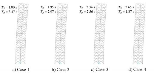
Figure 3. Fundamental mode of vibration for all versions of bracing sub-system
