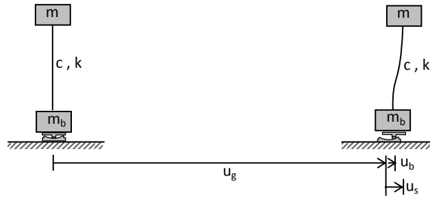
Figure 2. Mechanical Model of the Isolated Structure
