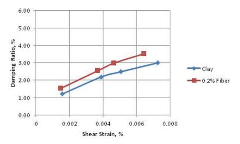
Figure 3. Damping ratio versus shear strain graph of clay and fiber reinforced clay
