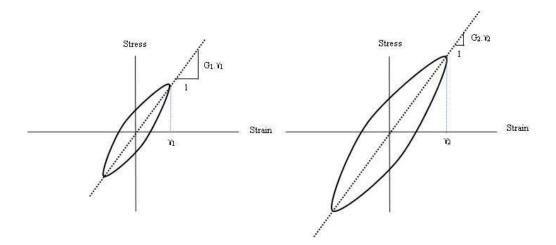
Figure 1. Stress-strain relationship in cyclic loading (Shannon and Wilson, 1972)
