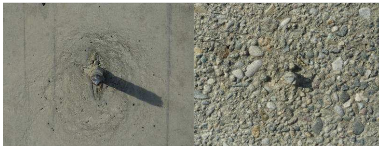
Figure 2.2. Specimens RCJ1 surface before and after sandblasting
