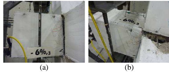
Figure 2.12. Damage in the secondary beam of specimen RCJ2 at the end of the test: (a) outer side of the joint; (b) inner side of the joint
