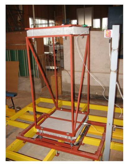
Figure 4. Base isolated single-storey model with two accelerometers and a laser displacement sensor
