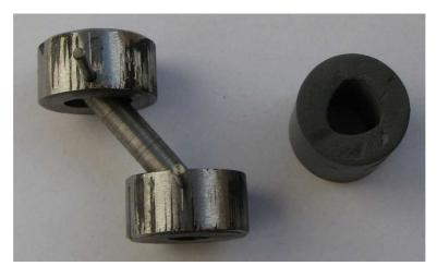
Figure 1. Prototype of the Elastomeric Polymer Bearing
