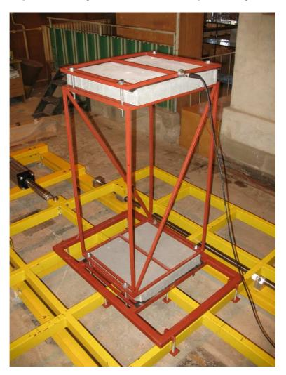
Figure 3. Non-isolated single-storey steel structure model mounted on the shaking table
