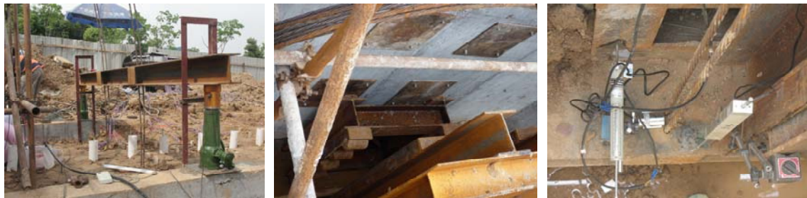
(a) Jacks for loading (b) The steel plate with cylinders (c) Displacement meters
