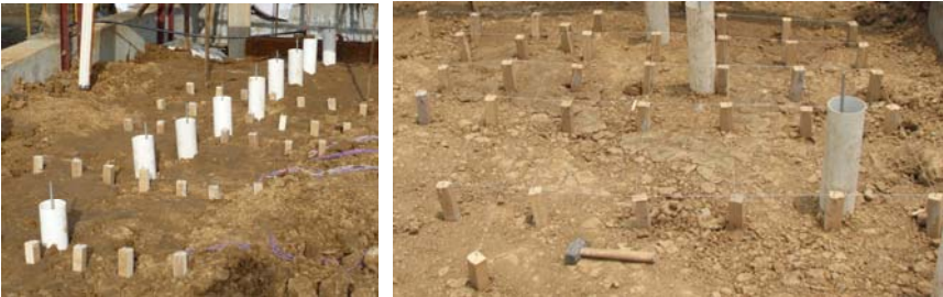
Figure 8. Small wooden stakes used for observation of the ground
