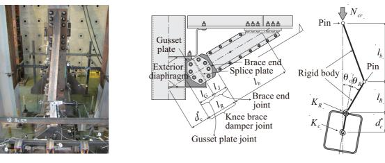
Figure 7. Out-of-plane buckling
