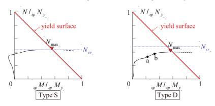
Figure 10. M-N interaction at splice plates of knee brace damper
