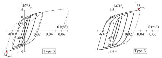
Figure 6. Bending moment at the beam end versus beam rotation angle relationship
