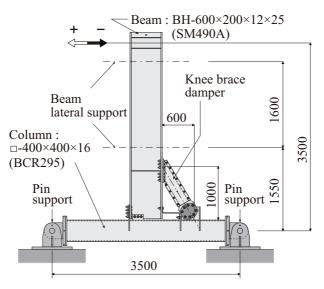
Figure 4. Test setup (unit: mm)
