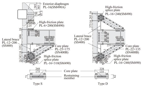
Figure 3. Details of beam-to-column connection (unit: mm)
