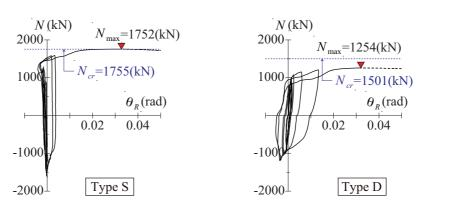
Figure 9. Axial force of knee brace damper versus rotational angle of brace joint relationship
