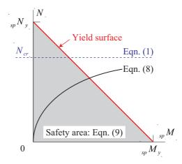
Figure 14. Design criteria of brace joint
