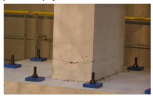
Figure 4.10. Damage to bridge pier base by T-I motion without dampers
