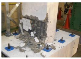
Figure 4.11. Damage to bridge pier base by T-II motion without dampers
