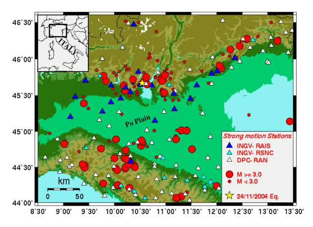
**Figure 1.1** INGV and DPC strong motion stations in Northern Italy and seismicity recorded by INGV-RAIS from June 2006 to March 2012. The yellow star indicates the 24<sup>th</sup> November 2004, M<sub>L</sub> 5.2, Salò earthquake.
