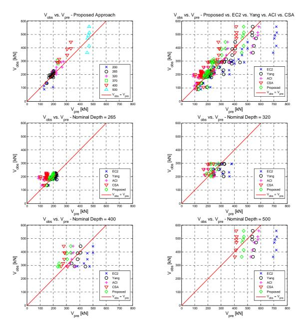
Figure 3.3 Proposed approach: experimentally observed,  $V_{obs}$ , vs. analytically predicted,  $V_{pre}$ , shear strength capacity, globally and separately compared with other analytical methods
