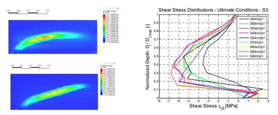
Figure 1.1 Comparison between principal tensile strain of circular (Specimen320c) and non-circular voids (Specimen320b) hollow core units and shear stress distributions close the support (x/D < 0.4)
