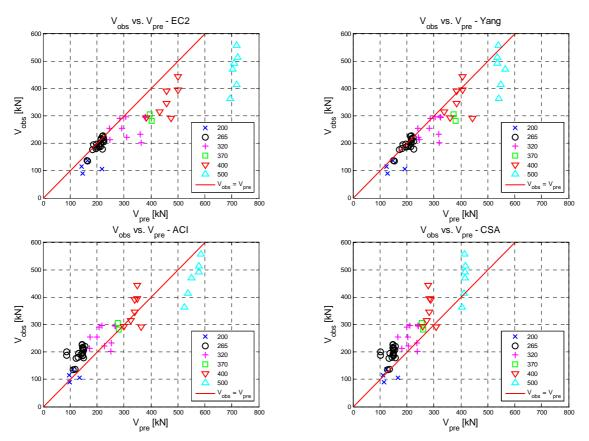
Figure 2.1 Experimentally observed,  $V_{obs}$ , vs. predicted,  $V_{pre}$ , shear strength capacity, for each nominal depth, according to EC2 provisions, Yang's design method, ACI and CSA recommendations, respectively
