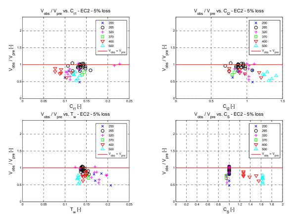
**Figure 3.1** Ratio between observed and predicted shear strength capacity,  $V_{obs}/V_{pre}$ , according to EC2 provisions and 5% loss of prestress ratio, vs. local cross-sectional geometric factors,  $C_{t1}$ ,  $C_{t2}$ ,  $T_w$  and  $C_s$ , respectively
