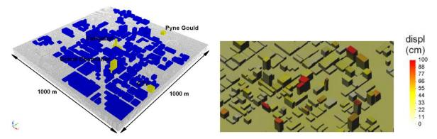
**Figure 2.1.** Left: 3D-model of the soil and the buildings in Christchurch CBD, Guidotti (2012) Right: Snapshots of the simulated displacement of the buildings of the Christchurch CBD, Guidotti (2012)
