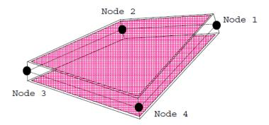
Figure 3.2. Shell4N element used to model the masonry structures in this study, SLang (2004)
