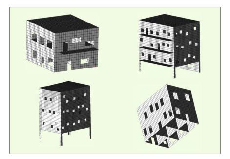
**Figure 3.3.** Four examples for the buildings Top left: Typical one family building with a small balcony Top right: Three storey building with balcony and soft storey Bottom left: Three storey building with soft storey Bottom right: View from bottom inside the building with the inner walls
