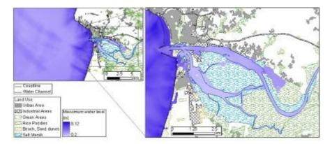
Figure 3.2. Maximum water level at Figueira da Foz.
