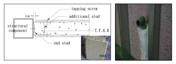
Figure 5. Details of the W6 specimen
