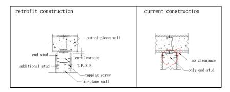
Figure 7. Retrofit construction in T shape wall
