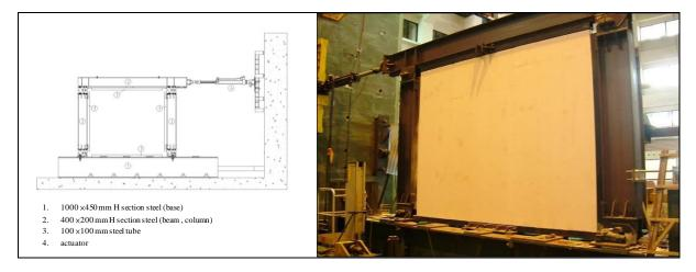
Figure 3. Details of the test frame
