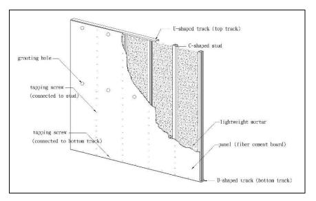
Figure 1. Typical construction of the DMF system
