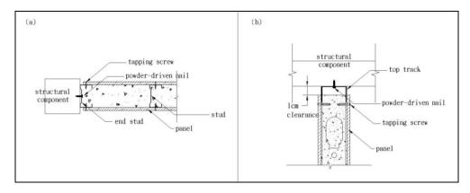
Figure 2. Details of the end stud (a) and the top track (b)
