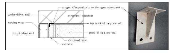
Figure 8. Details at the top junction of two walls in W8 specimen
