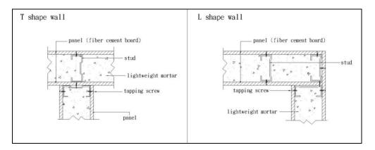
Figure 4. Detailed connections of the T shape wall and the L shape wall
