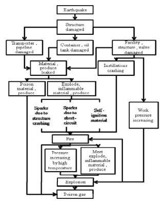
Figure 2.1. Sketch of earthquake disaster chain in petrochemical industry system
