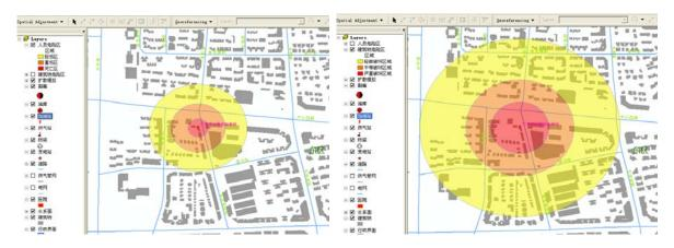
Figure 5.1. Coverage of casualties (left) and coverage of building damaged (right) after explosion
