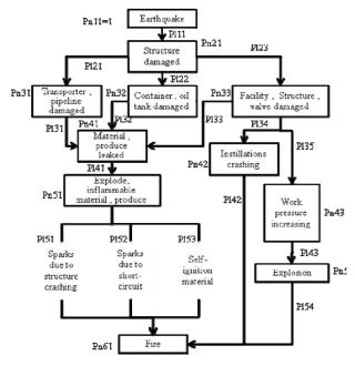
Figure 2.2. Earthquake & fire links in disaster chain of petrochemical industry system
