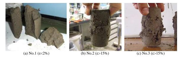
Photograph 2. Failure conditions of specimens after unconfined compression test
