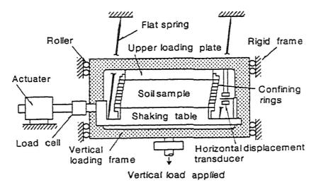
Figure 1. Schematic view of cyclic simple shear testing apparatus
