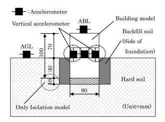
Figure 11. Accelerometer layout sketch
