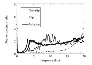
**Figure 12.** Fourier spectrum ratios ( $\ddot{\theta}$ H /AGL)
