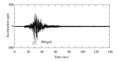
Figure 7. Acceleration time history and maximum acceleration of KOKUJI wave (JMA Kobe phase)
