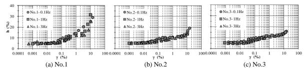
Figure 4. Damping ratio vs. shear strain
