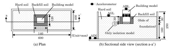
Figure 5. Plan and sectional side view of the experimental model
