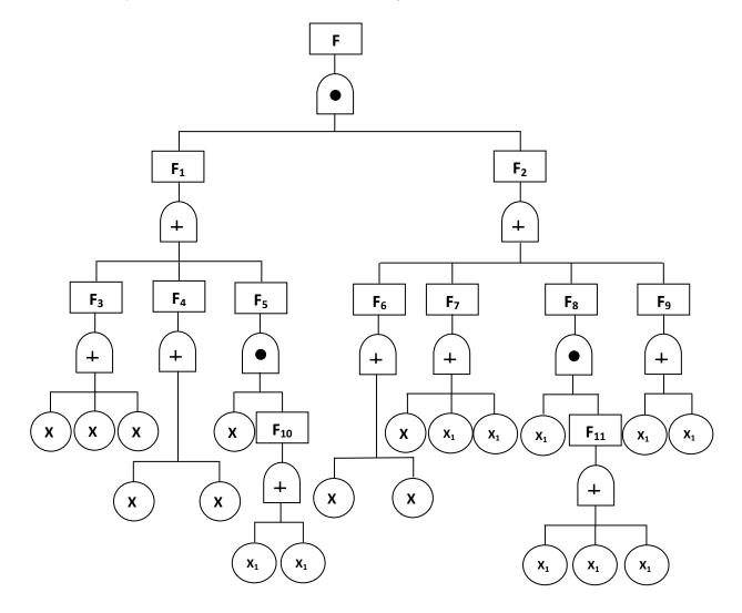
Figure 1. Fault tree diagram of storage tank secondary fire
