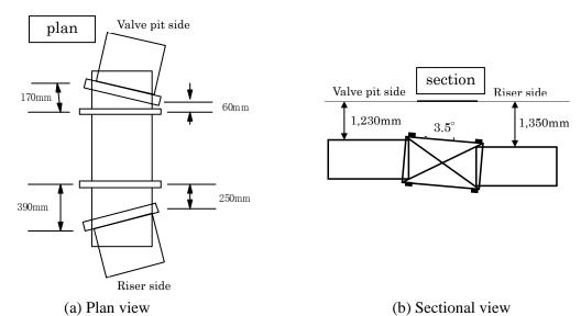
Figure 3.10. Site allocation of expansion joint after leakage
