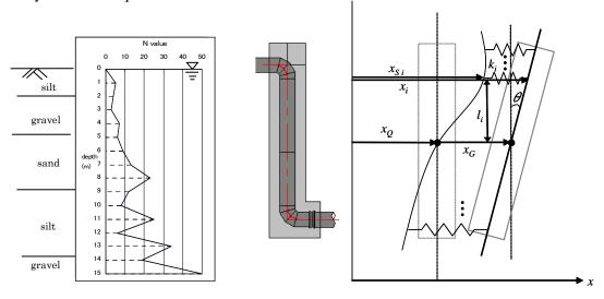
Figure 3.11. Soil classification and N value at site Figure 3.12. Configuration of the coordinate system for riser
