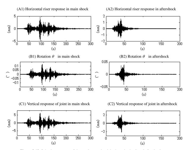
Figure 3.13. Seismic responses of riser and expansion joint in main shock and aftershock
