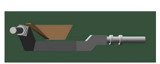
**Figure 3.2.** Three-dimensional illustration of under-crossing concrete encased structure
