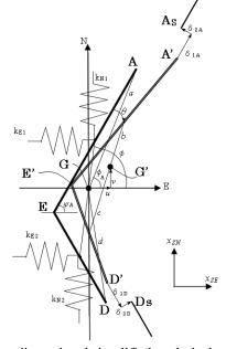
**Figure 3.3.** Two-dimensional simplified analytical model of under-crossing concrete encased structure
