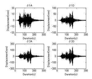
Figure 3.4. Excessive displacement between structural response and ground displacement at expansion joint points A and D, where  $\delta_1$  is axial displacement and  $\delta_2$  is transverse displacement to the pipe axis
