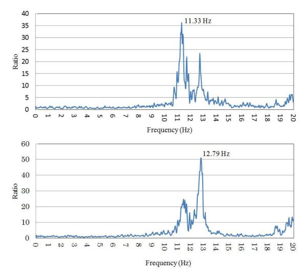
Figure 3. Transfer function of ambient vibration measurements
