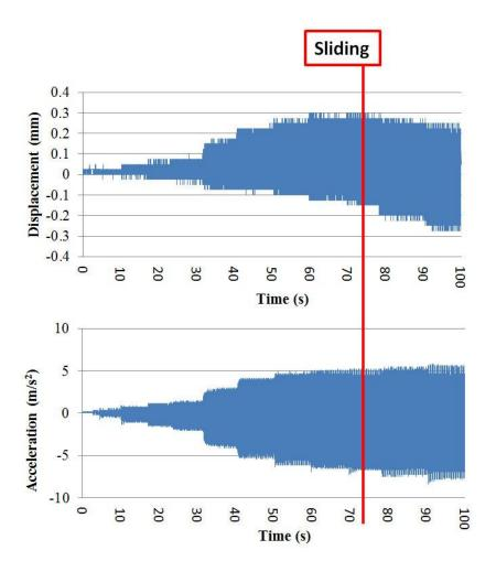
Figure 5. Detection of the sliding and corresponding acceleration for estimation of friction coefficient
