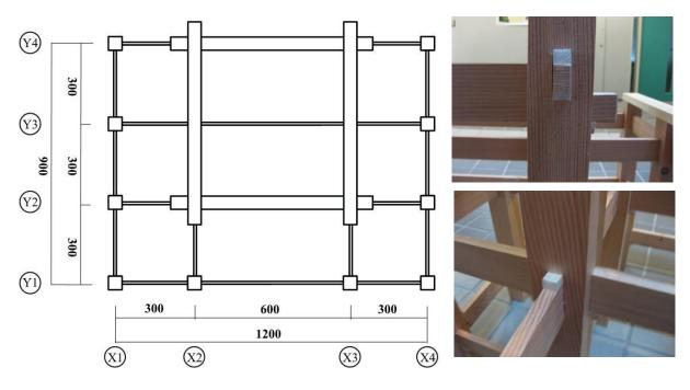
Figure 2. Dimension of the model and joint details
