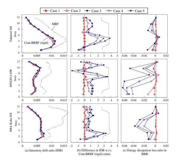
Figure 4.4. Deformation and energy dissipation results
