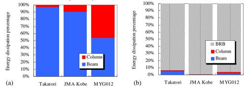
Figure 3.2. Hysteretic energy dissipation distributions among different components: (a) moment resisting frame (MRF) and (b) continuously buckling restrained braced frame
