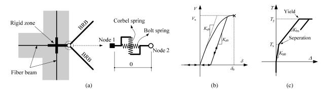
Figure 4.1. Modeling of BRB connections: (a) bi-axial spring element, (b) hysteresis of a single corbel and (c) force-displacement relationship of bolt spring
