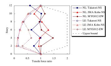
Figure 3.4. Maximum horizontal force in BRB connections
