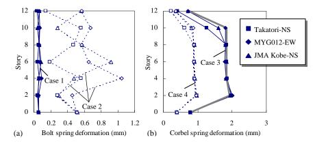
Figure 4.3. Maximum bolt spring deformations
