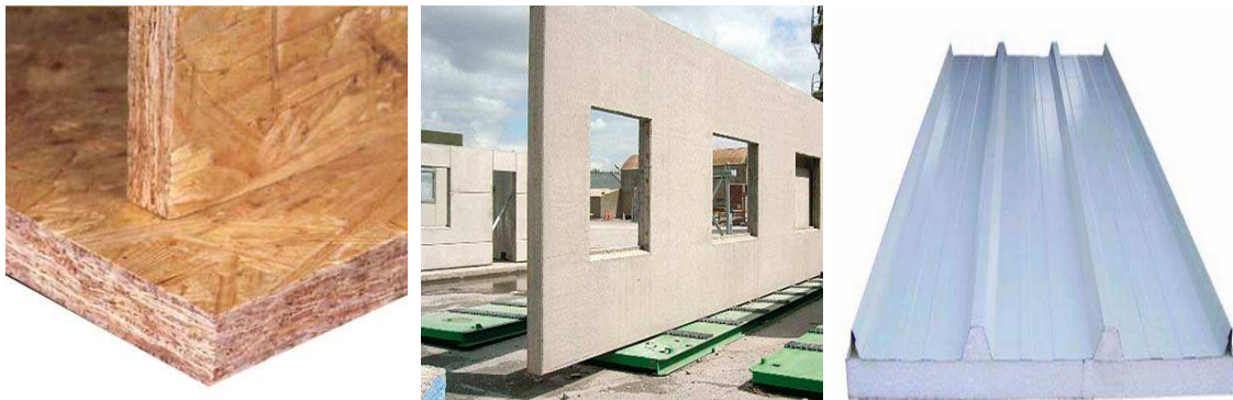
Figure 1.1. Typical panels; (a) OSB; (b) precast concrete; (c) metal, after Mashal, (2011)
