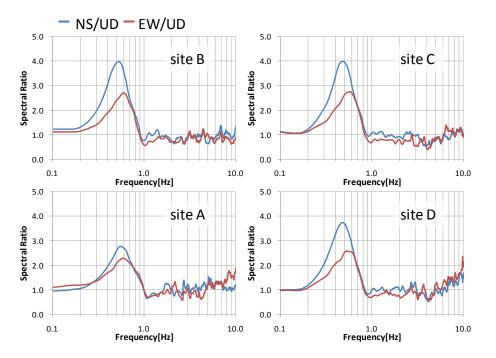
Figure 2.2. Average H/V spectral ratio of June 21st, 2010, observed at sites A to D in Fig. 2.1b
