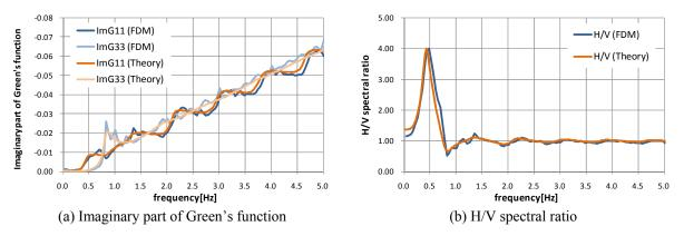
Figure 4.2. Comparison of (a) imaginary part of Green's function and (b) H/V spectral ratio of theoretical and numerical results for 1-D velocity model in Table 4.2
