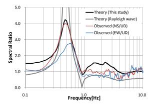
**Figure 3.2.** Theoretical H/V spectral ratio (black line) compared against H/V spectral ratio derived from ellipticity of Rayleigh waves (gray line) and observed H/V spectral ratio of June 21st, 2010 (red and blue lines)
