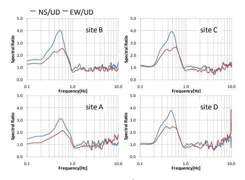
Figure 2.3. Average H/V spectral ratio of June 23<sup>rd</sup>, 2010, observed at sites A to D in Fig. 2.1b
