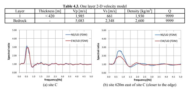
**Figure 4.3.** Comparison of H/V spectral ratio of NS/UD and EW/UD at (a) site C and (b) site 620m east of site C closer to the edge, calculated by FDM for 2-D basin model
