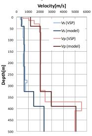
Figure 3.1. Velocity profile from VSP survey near site C (light lines) and assumed 1-D velocity model with 3 layers (dark lines)
