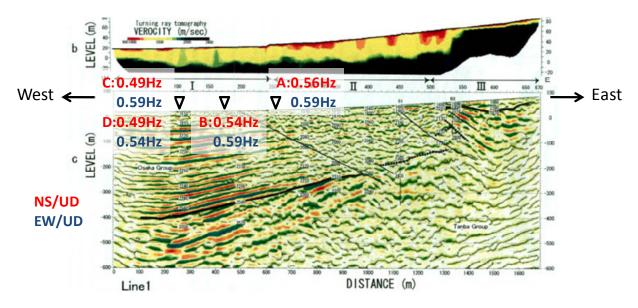
Figure 2.4. Section profile beneath Uji campus along the east-west survey line in Fig. 2.5b (After Koizumi *et al.*, 2002) and peak frequencies of average H/V spectral ratios of June 21<sup>st</sup>, 2010, observed at sites A to D in Fig. 2.1b
