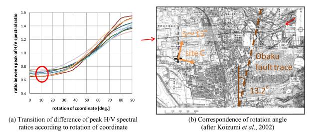
Figure 2.5. Correspondence of rotation angle for lowest difference of peak H/V spectral ratio to the Obaku fault just east of Uji campus
