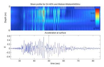
Figure 1. Colormap of Induced Shear Strain vs. Depth and Time (upper plot) and Recorded Ground Surface Accelerogram (lower plot) in Model Tested in the NEES at Rensselaer Polytechnic Institute (RPI) Centrifuge
