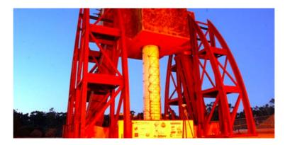
Figure 2. Full-scale Bridge Column on the University of California, San Diego NEES@UCSD Shake Table
