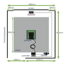
Figure 5. Appearance of earthquake simulation system
