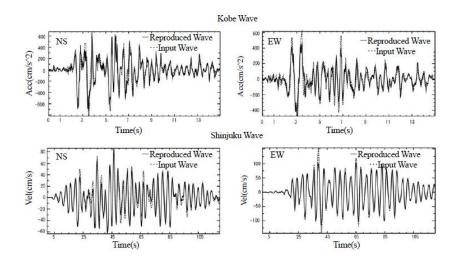
Figure 4. Comparison between input earthquake motions (dotted line) and the earthquake motions reproduced by Jishin The VUTON (solid line)
