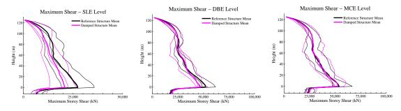
Figure 9.4 Maximum Storey Shear – North-South Direction
