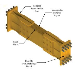
Figure 2.1 Viscoelastic Coupling Damper (VCD)
