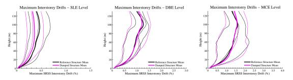
Figure 9.2 Maximum Interstorey Drifts - North-South Direction
