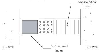
Figure 4.1 Shear force limiting VCD
