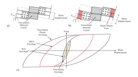
Figure 2.2 a) Viscoelastic deformed shape, b) Viscoelasto-plastic deformed shape, c) Design hysteresis envelopes
