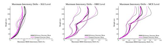
Figure 9.1 Maximum Interstorey Drifts - East-West Direction
