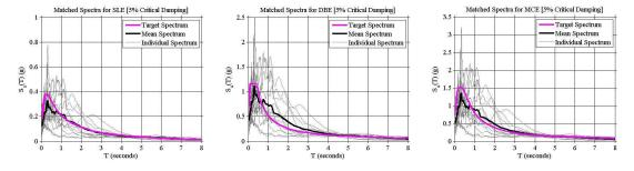
Figure 6.1 Scaled site specific spectra
