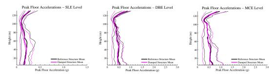
Figure 9.5 Maximum Storey Acceleration - East-West Direction
