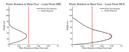
Figure 9.8 Peak Shear Fuse Plastic Rotations - Loma Prieta
