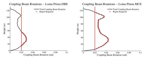
Figure 9.7 Peak Coupling Beam Rotations - Loma Prieta
