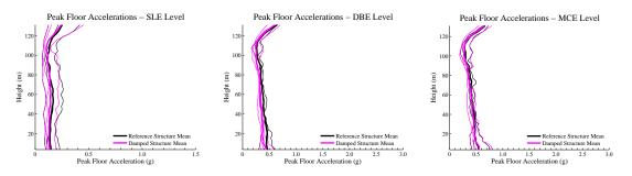
Figure 9.6 Maximum Storey Accelerations - North-South Direction
