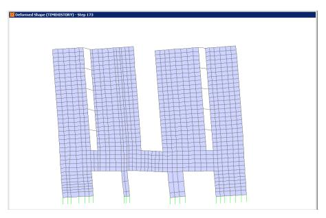
Figure 3. Deformed shape of coupled shear walls on Line 7 showing uplift
