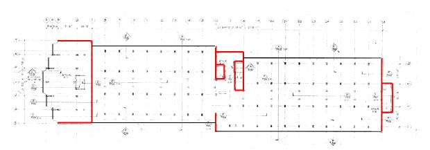
Figure 1. Typical floor plan showing shear wall locations in red
