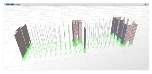
Figure 3. Computer model of building without slabs to show locations of shear walls
