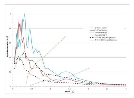
Figure 4. Rayleigh period shift of building shown versus recorded and damped response spectra
