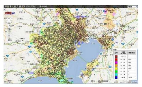
Figure 3. SI value observed by SI Sensors and Interpolated SI Values by 50m Meshes
