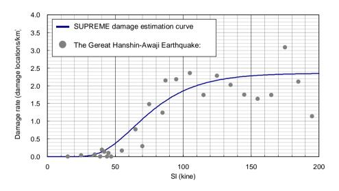
Figure 2. Damage Estimation Curve of SUPREME
