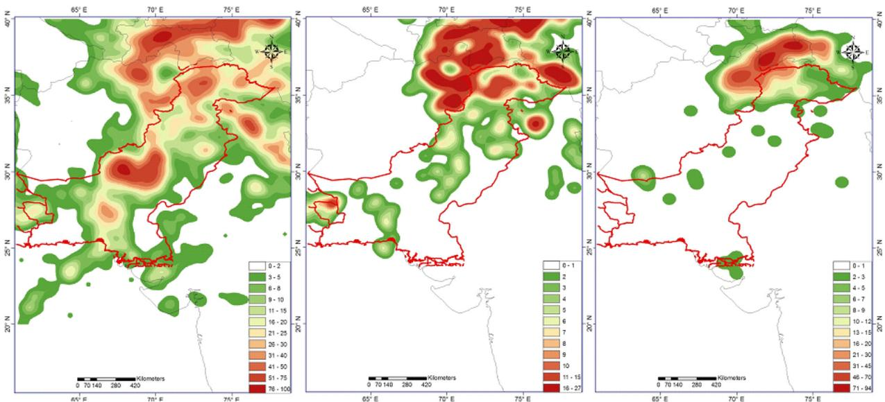
**Figure 5.** Smoothed activity rate  $10^a$  value derived for seismicity from 0-50km, 51-100 km and 101- 250 km depth
