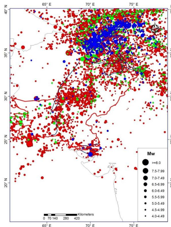
**Figure 3.** Pakistan and its surrounding seismicity from 1902 to 2009; red: 0-50 km depth, green: 51-100 km depth, and blue: 101-250 km depth
