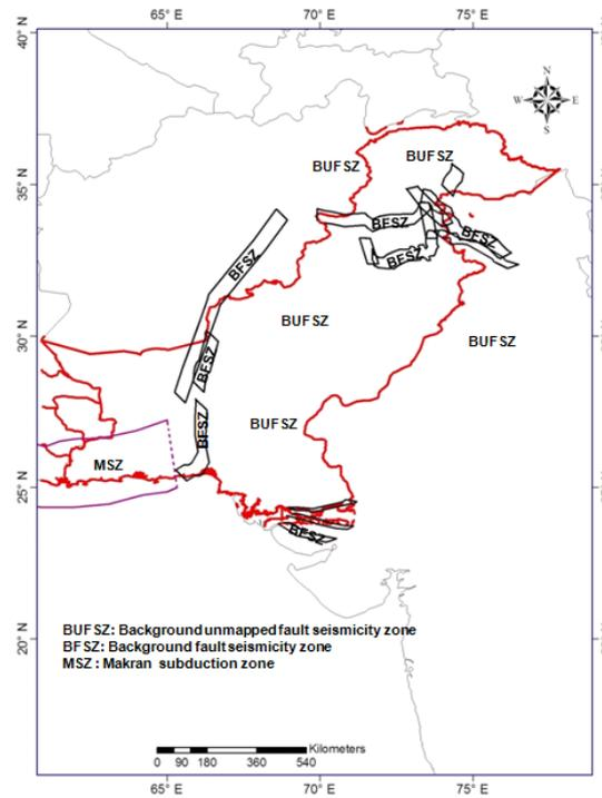
**Figure 4.** Earthquake sources of the study area: Background unmapped fault seismicity zone (BUFSZ), Background fault seismicity zone (BFSZ), and Makran subduction zone (MSZ)
