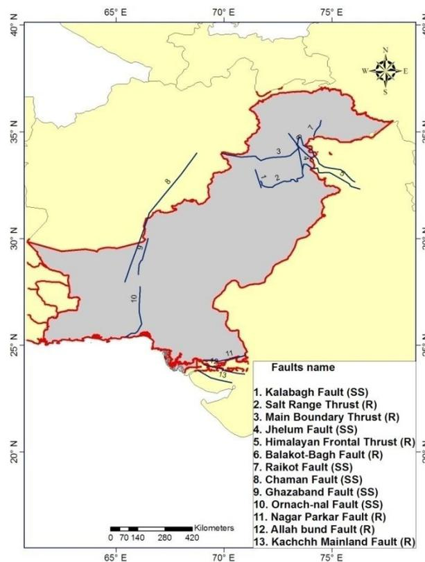
**Figure 6.** Thirteen crustal fault source models incorporating in this study (SS: Strike-Slip fault, R: Reverse fault)
