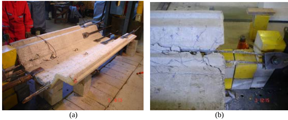
Figure 3.1. Monotonic tension loading tests of bars embedded into the Dalla-beams: (a) Arrangement; (b) Typical failure mode of Dalla-beams specimens provided by Preansa S.A.
