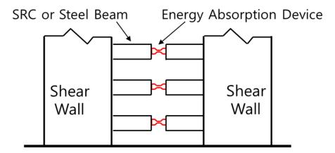
**Figure 1.** Location of Coupling Beam Proposed in this Study
