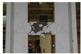
(c) Coupling Beam – Front (d) Coupling Beam - Back **Figure 9.** Damage Status of ECS Specimen
