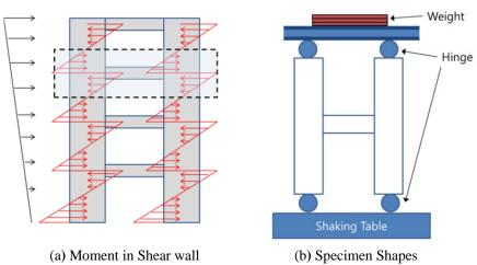
Figure 3. Test Specimen Shapes
