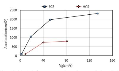
Figure 7. The Relation between acceleration and energy-equivalent velocity
