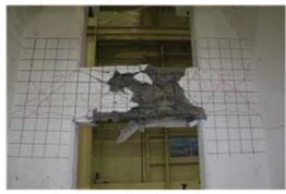
(b) Shear Wall and Coupling Beam
