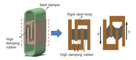
Figure 2. Shape of Hybrid Energy Dissipative Device
