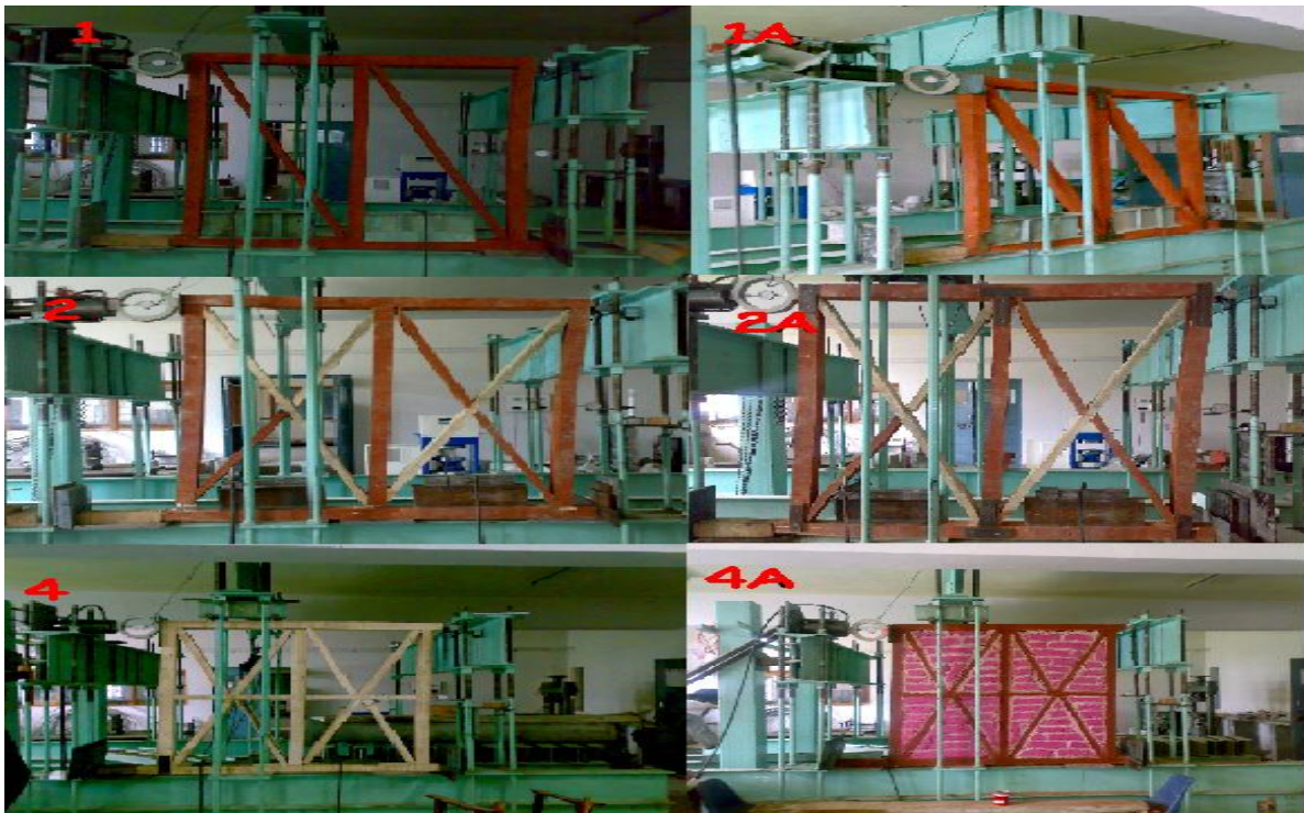
Figure 2. Test samples under test,on the Loading Frame
