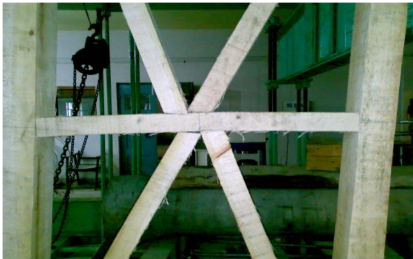
Figure 8. Bending induced in Bracings of Frame 4
