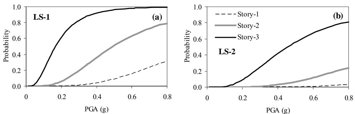
**Figure 3.1.** Fragility curves for a typical three story URM building with RC floor slab (nearly fixed boundary conditions) according to the story number where the critical face-loaded wall is located and for a) LS-1, b) LS-2
