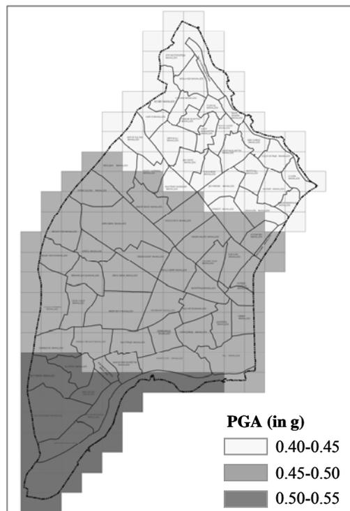
**Figure 4.1.** Grid by grid distribution of PGA values in terms of g for an event with a return period of 475 years in Fatih sub province.
