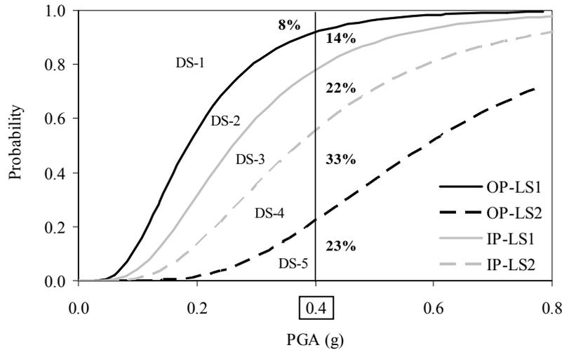
**Figure 4.2.** Demonstration of VS calculation by using the fragility curves (both for IP and OP response) of the selected masonry building type
