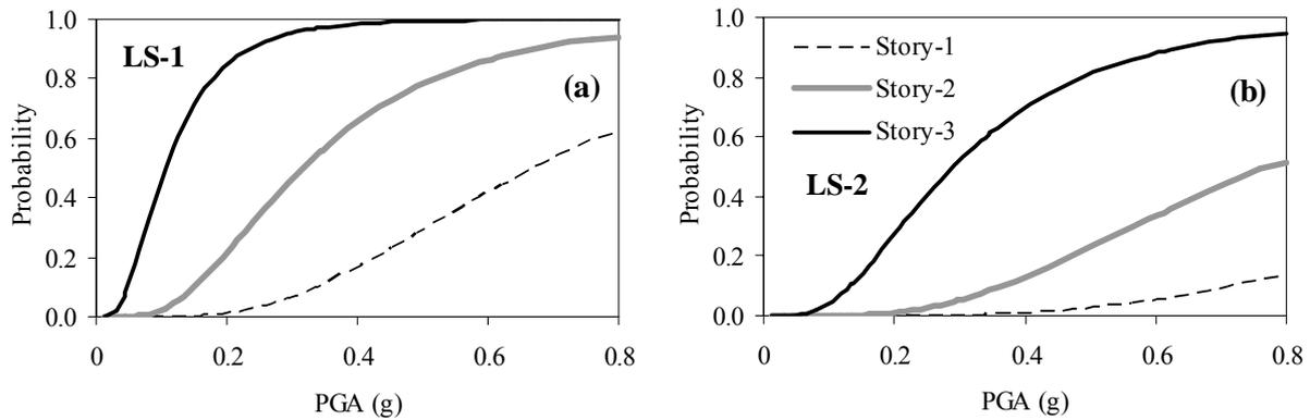
**Figure 3.2.** Fragility curves for a typical three story URM building with wooden floor slab (nearly hinged boundary conditions) according to the story number where the critical face-loaded wall is located and for a) LS-1, b) LS-2
