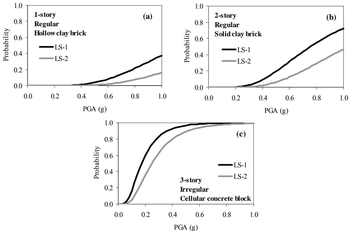
**Figure 2.1.** Typical fragility curve sets for in-plane behaviour of (a) a single story, regular masonry building with moderate quality hollow clay brick units; (b) a two story, regular masonry building with moderate quality solid clay brick units; (c) a three story, irregular masonry building with poor quality cellular concrete blocks.
