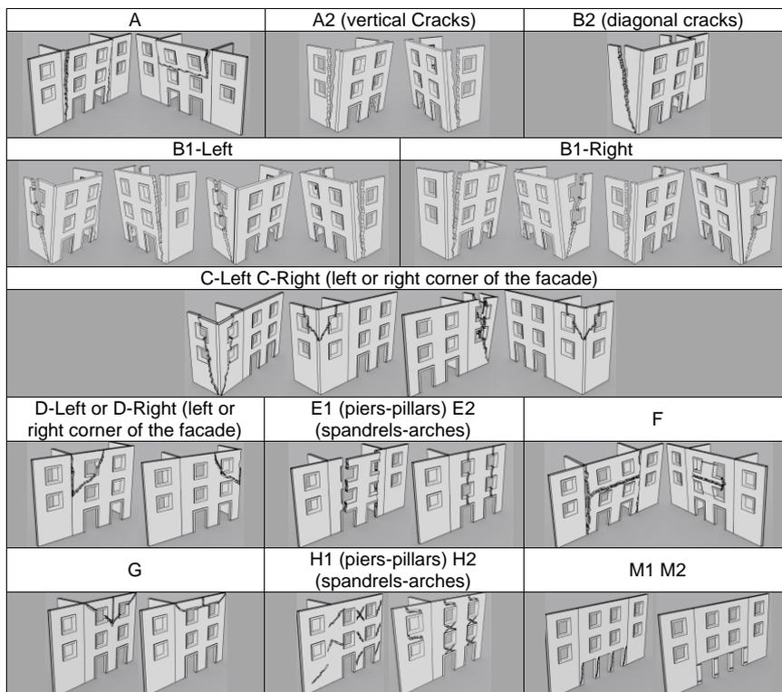
**Figure 6-1** Collapse mechanisms
