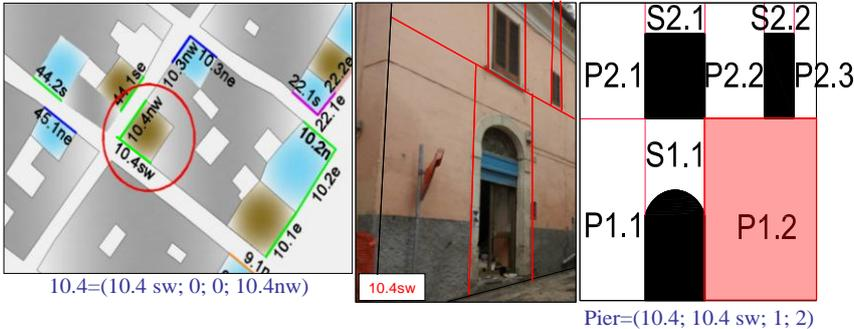
**Figure 3-3** Structural enumeration convention of the façade 10.4sw
