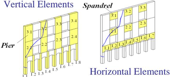
**Figure 3-2** Correlation Identification and naming of the structural elements of a façade
