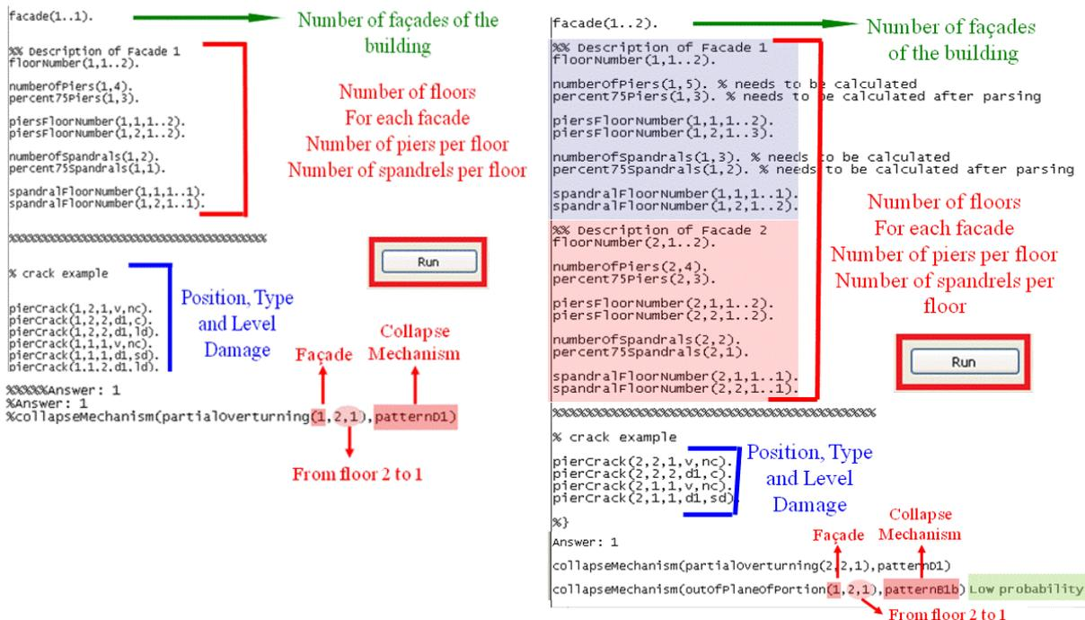
Figure 6-2: LOG-IDEAH applied a) on the façade 22.1e and b) on both façades 22.1e and 22.1s
