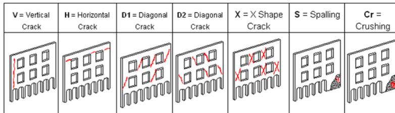
**Figure 4-1** Structural damage types
