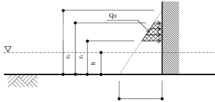
**Figure 1.** Japanese design guideline for tsunami evacuation building 2005 ( $a=3.0$ )
