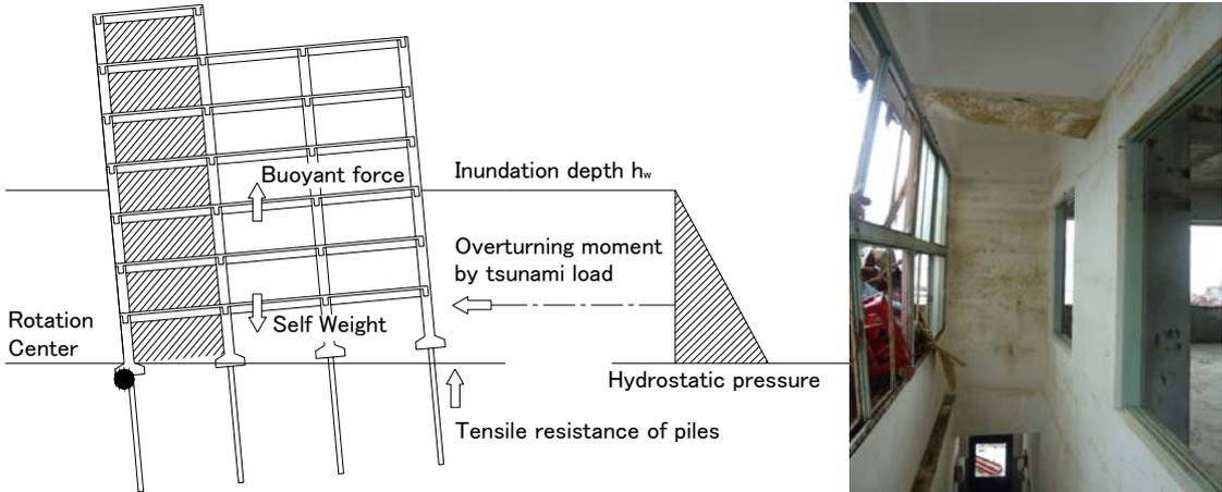
(a) Overturning mechanism of the building (b) Inside of a survived building
