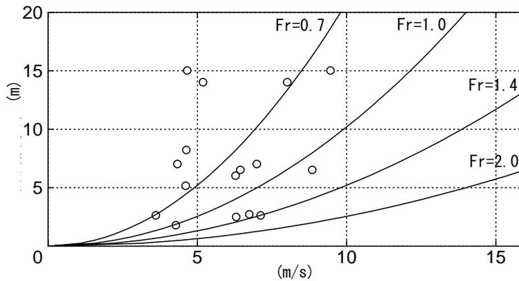
**Figure 2.** Comparison between inundation depth and flow velocity in several regions
