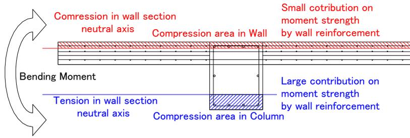
**Figure 6.** Calculation of out of plain bending moment strength for variable cross section
