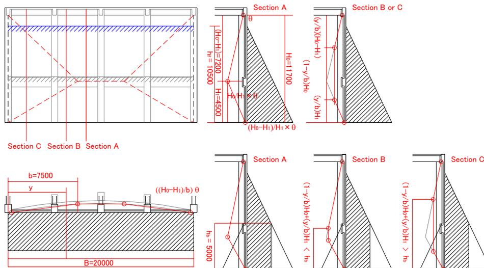
**Figure 5.** Plastic hinge mechanism on damaged frame
