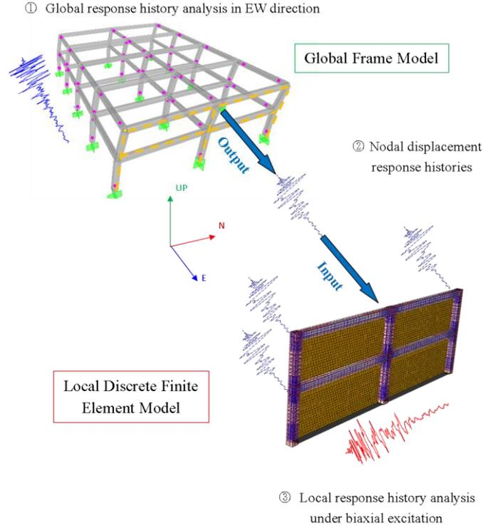
**Figure 2.2** Schematic diagram of modelling and analysis procedure
