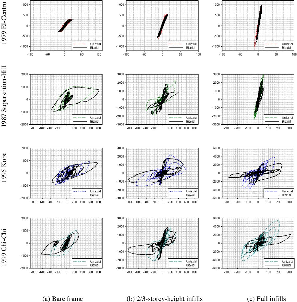
**Figure 4.1.** In-plane (NS-direction) hysteresis loops of infilled RC frames under four ground-motion histories (vertical axis: base shear (kN); horizontal axis: top drift (mm))
