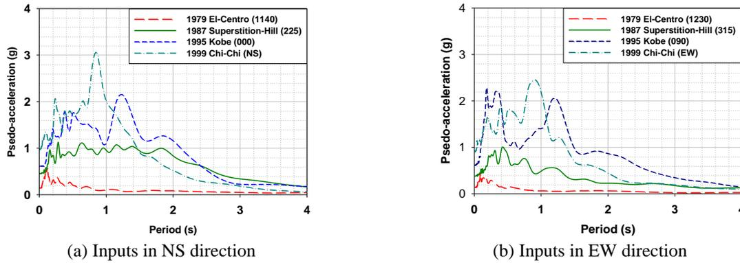
**Figure 3.2.** Elastic response spectra of ground-motion histories
