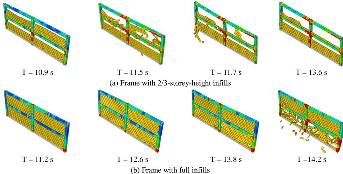
**Figure 4.3.** Progressive collapse of infill walls under biaxial excitation of 1999 Chi-Chi earthquake
