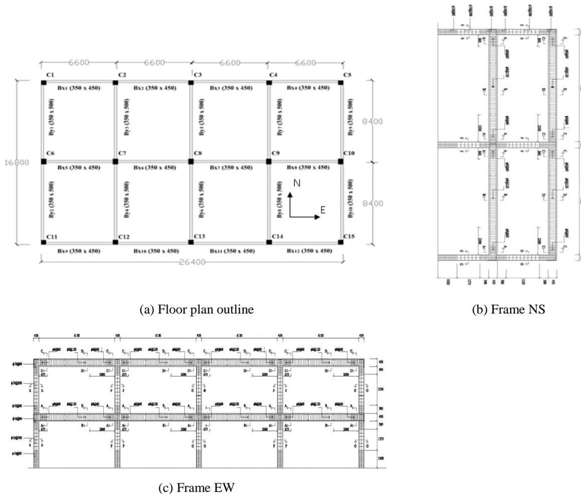
**Figure 2.1.** Dimensions and reinforcement details of prototype RC structure (mm)
