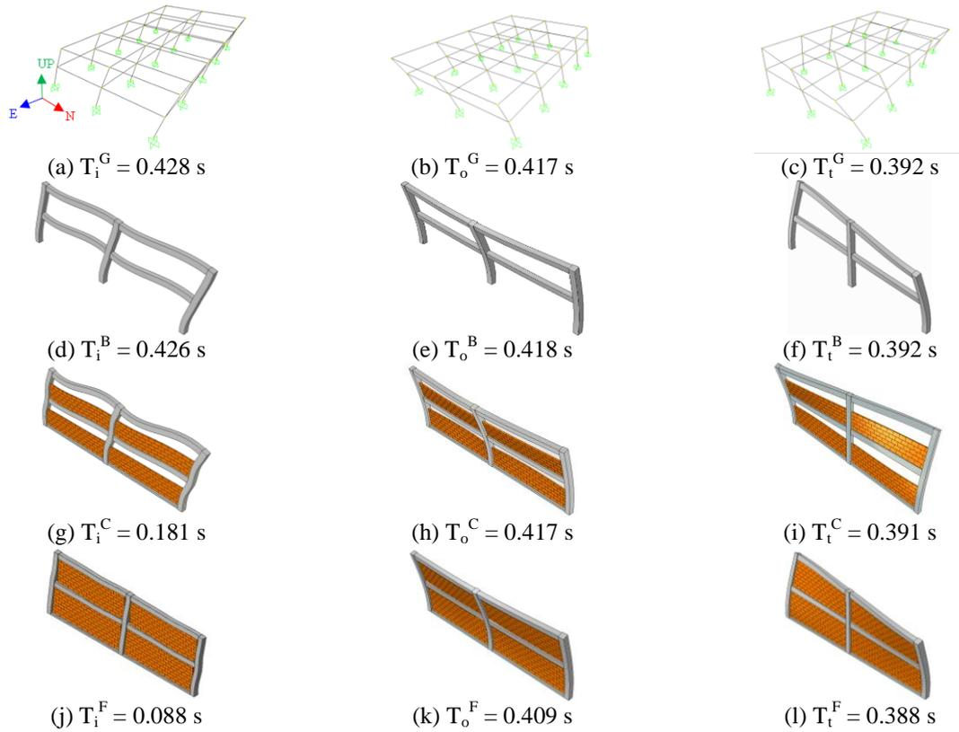
**Figure 2.3.** Natural vibration modes of the global and local frames (mass-springs are hidden for simplicity)
