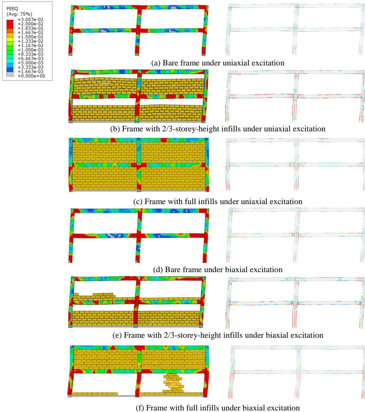
**Figure 4.2.** Damage pattern of the infilled RC frame structures ( $t = 14.1$  s) under 1999 Chi-Chi earthquake (contour-plot of equivalent plastic-strain)
