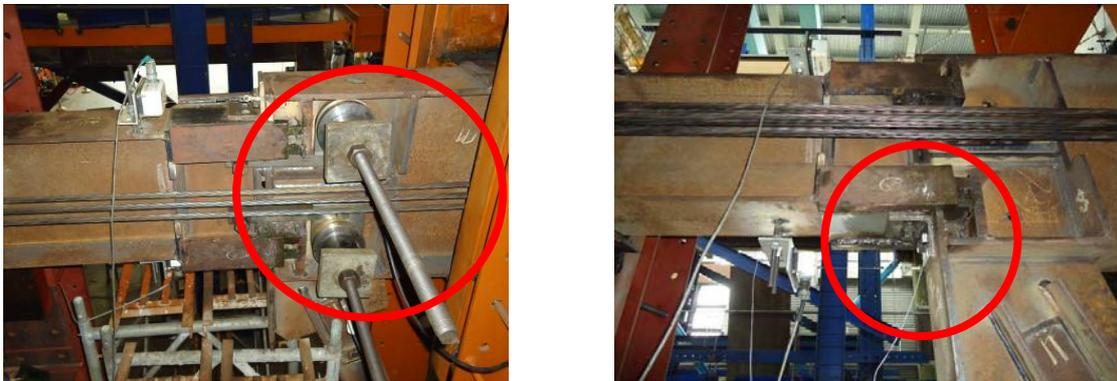
Figure 1. Left photo shows the frictional hinge damper and right photo shows steel angles installed
