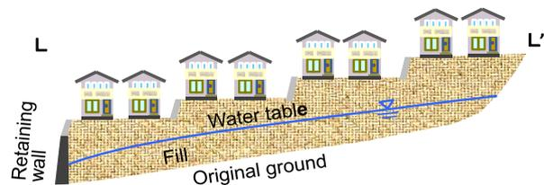
Figure 2 Typical soil cross section in filled ground
