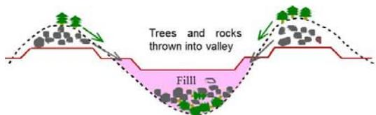
**Figure 5** Procedure of reclamation work conducted at Midorigaoka
