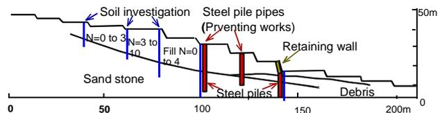
**Figure 6** Soil cross section along failed slope (Tohoku Branch, JSCE)
