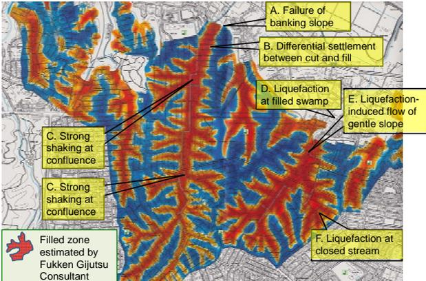
**Figure 13** Six damage patterns observed at Nankodai in Sendai City
