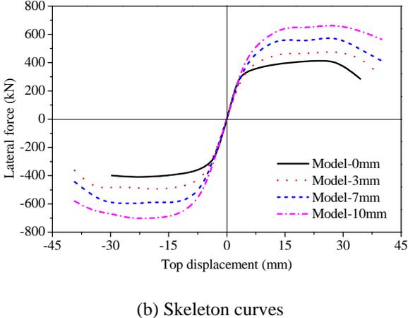
**Figure 3.4.** Load-displacement curves for different thickness of steel plate
