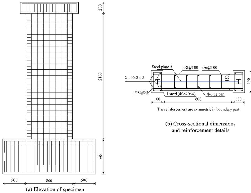
**Figure 2.1.** Elevation of specimen and cross-sectional views and reinforcement details (unit: mm)
