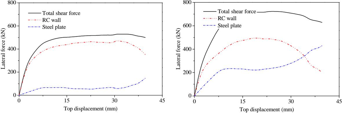
**Figure 3.5.** Load-displacement responses for RC wall and steel plate
