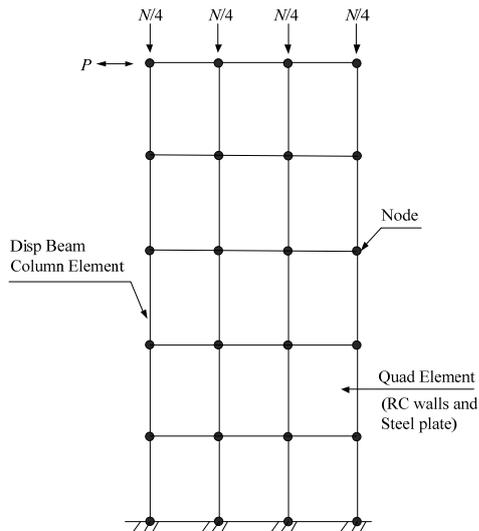
**Figure 2.2.** Finite element modelling of specimen
