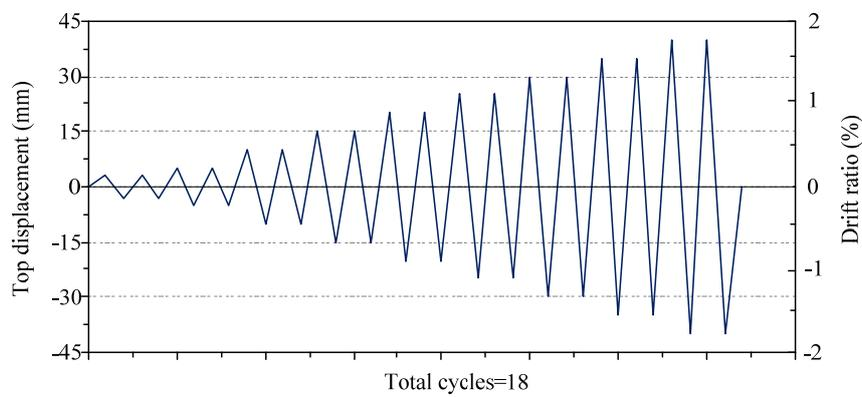
**Figure 3.1.** Top lateral displacement history of all analytical models
