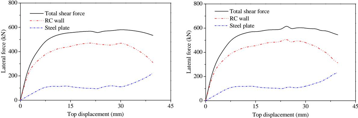
(a) 0.2% web reinforcement (b) 0.8% web reinforcement
