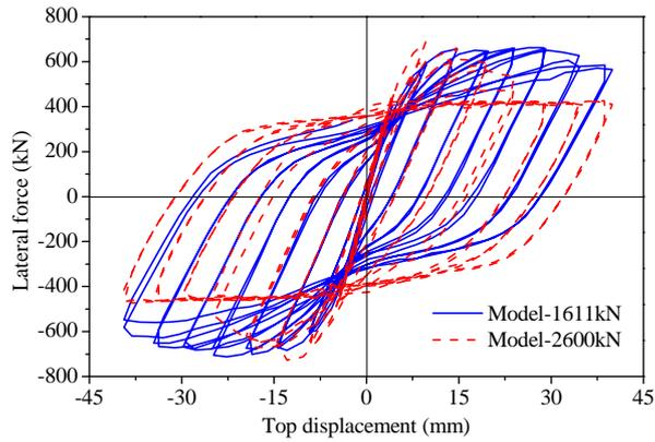
**Figure 3.6.** Load-displacement responses for different vertical loads with 10mm steel plate
