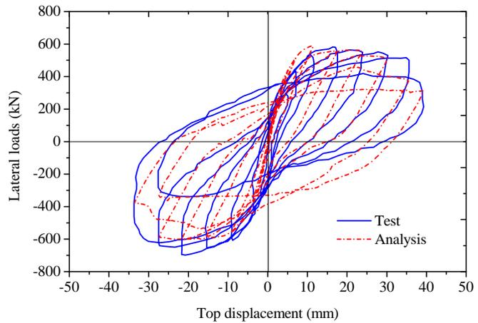
**Figure 2.3.** Analytical and test load-displacement curves
