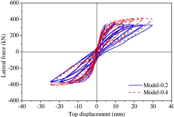
**Figure 3.8.** Load-displacement curves for conventional RC walls with different web reinforcement
