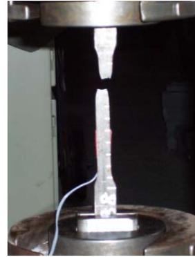
**Figure 1.** Average stress-strain curve and failure view of one coupon
