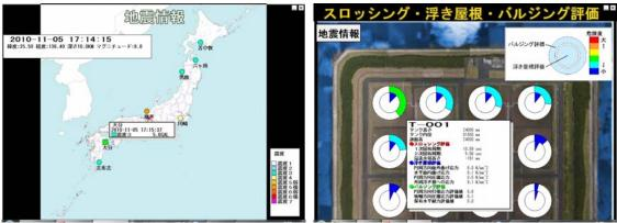
(a) Seismic intensity of an object sites(b) Example of Tank DamageFigure 3.3 Example of an evaluation result display screen
