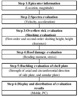
Figure 3.1 Tank damage evaluation flow
