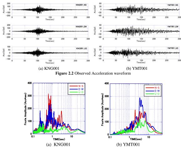
Figure 2.3 Comparison of an acceleration Fourier spectrum at two sites
