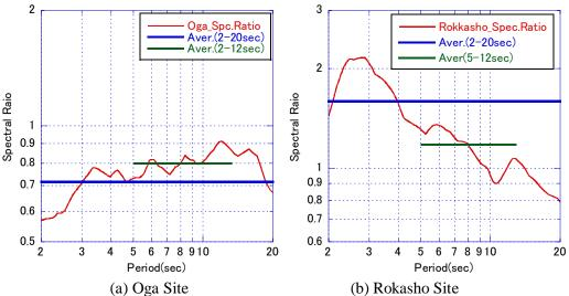
Figure 4.2 The acceleration response spectral ratio to the Akita and the Hachinohe meteorological observatories
